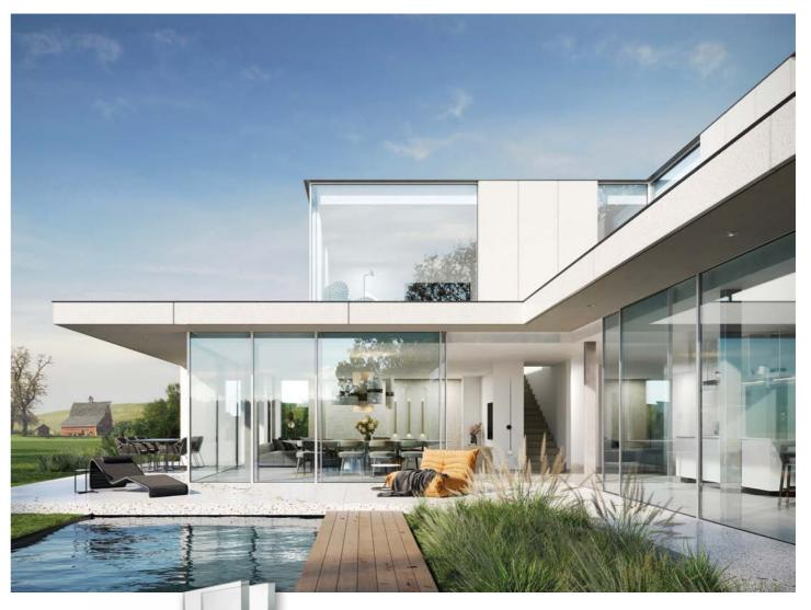
Thanks to the fully integrated ultra-slim profiles, transparency is maximised. This system is **completely barrier-free** and regulates drainage with a sloping pedestal profile connected to a drainage channel on the outside of the sliding window.
